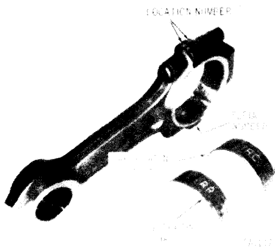
Figure 3-170. Connecting rod and bearing location number.
