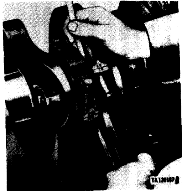
Figure 3-176. Checking connecting rod side clearance.
