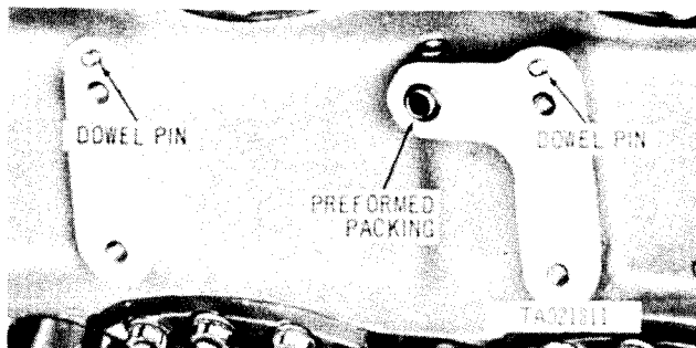
Figure 3-87. Location of preformed packing at oil transfer tube for fuel injection pump mounting base.
